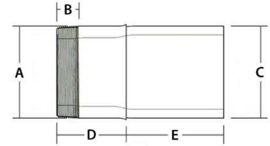
**SDR 17** (Standard Dimension Ratio) 125 PSI (Working Pressure at 73.4° F)
