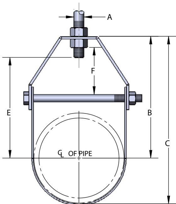
“E” dimension includes exposed rod threads beyond bottom of the hex nut. Exposed rod thread dimension is equal to the diameter of the rod used.
