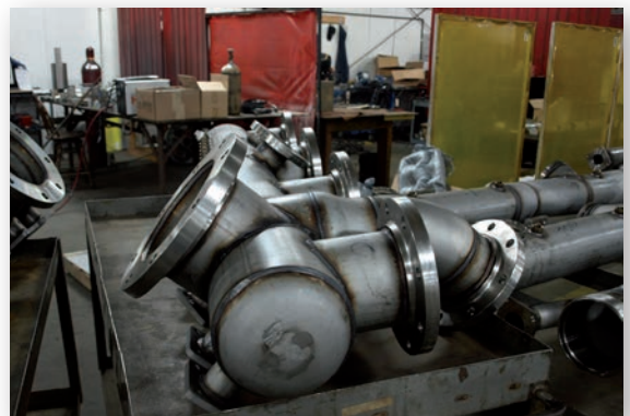
Stainless Steel Mixing Stations awaiting pressure testing
